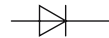
Figure 28.72: Switching diode: circuit symbol and typical characteristic values V_S : low (Si: 0.7 V, Ge: 0.3 V), V_Z : 50 ... 100 V, I_F : 50 ... 200 mA, I_R : \approx 1 nA, \tau : 2 ... 20 ns.
